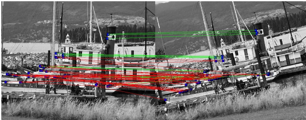
Fig. 3: A correspondence between the first two images of the BOAT sequence with the correct (green) and incorrect (red) mappings generated by the Match-Features functions contained in Matlab.
