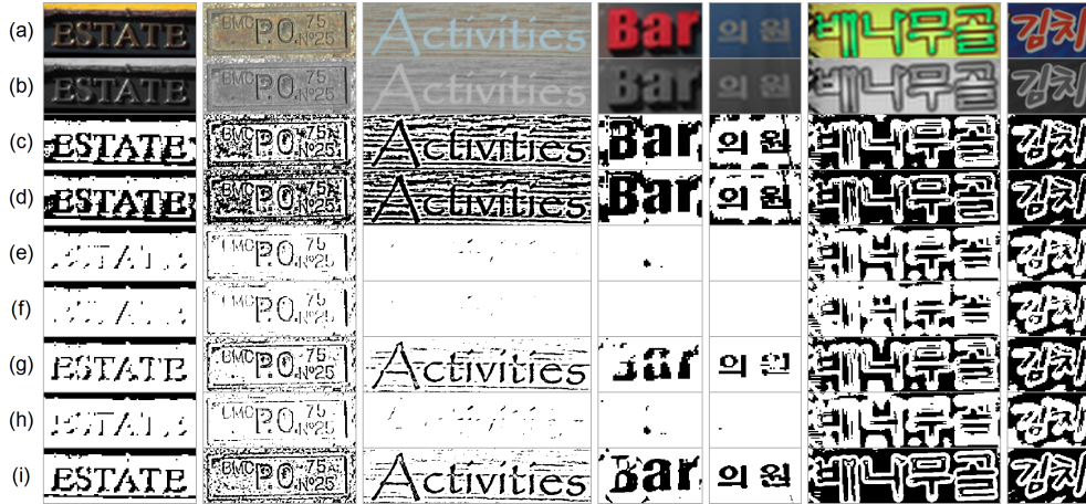
Fig. 3. Comparison of local binarization methods. (a) Source image, (b) Niblack [11], (c) Bernsen [1], (d) Sauvola and Pietikinen [13], (e) Wolf et al. [15], (f) Bradley and Roth [2], (g) NICK [7], (h) Proposed method.
