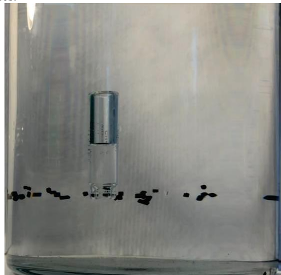
Figure 1 - A small glass bottle partially filled floats in equilibrium inside a density stratified liquid. Small plastic fragment with a known density are localized at a height where their density is matched and allow visualizing the internal gravity waves originated by the diver's oscillations.
