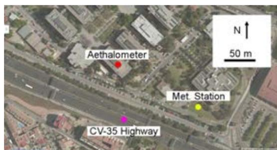
Fig. 1. Map of the measuring site showing the location of the Aethalometer (red), the meteorological station (yellow) and the CV-35 highway (pink). Copyright: 2014 Microsoft Corporation.
